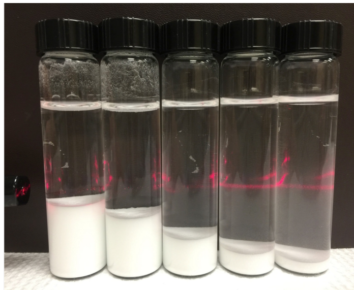
Figure 3-5 Equilibrated calcite dispersions ( \text{Na}_2\text{CO}_3 , I=0.1 M), Settling for 60 min, Laser coming from left
